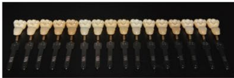
By use of series of colored raw materials, Self-Glazed Zirconia Restorations could precision reproduce the 16 color effects according to Classic Vita shade guide through completely digital manufacturing way.
