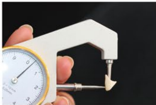
Ultra-thin Self-Glazed Zirconia dental crown (0.3 mm) made by net-shape manufacturing.
